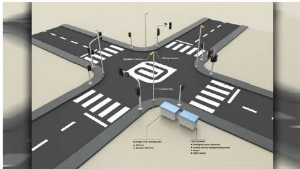
Dynamic Intersection (Intelligent Traffic) Management System
